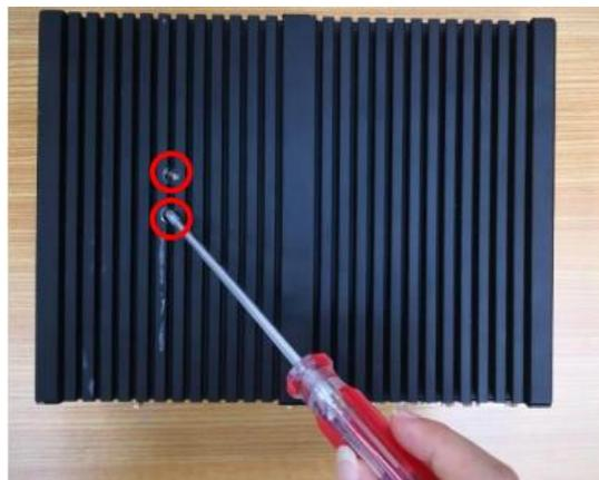
3. Remove the 2 screws in the marked spots with a screwdriver.
