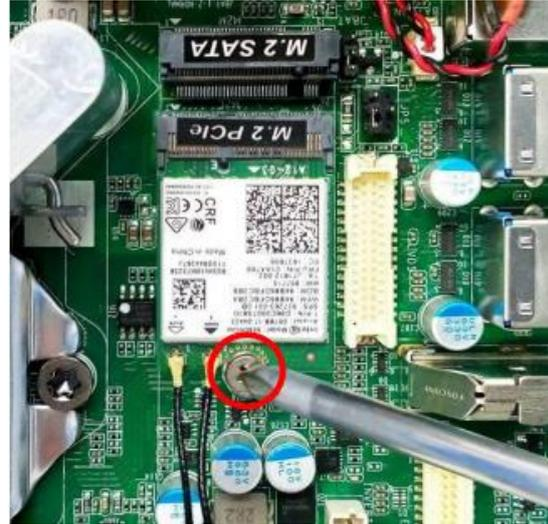
2. Remove the marked screw fixed on the screw post for M.2 SATA card installation.
