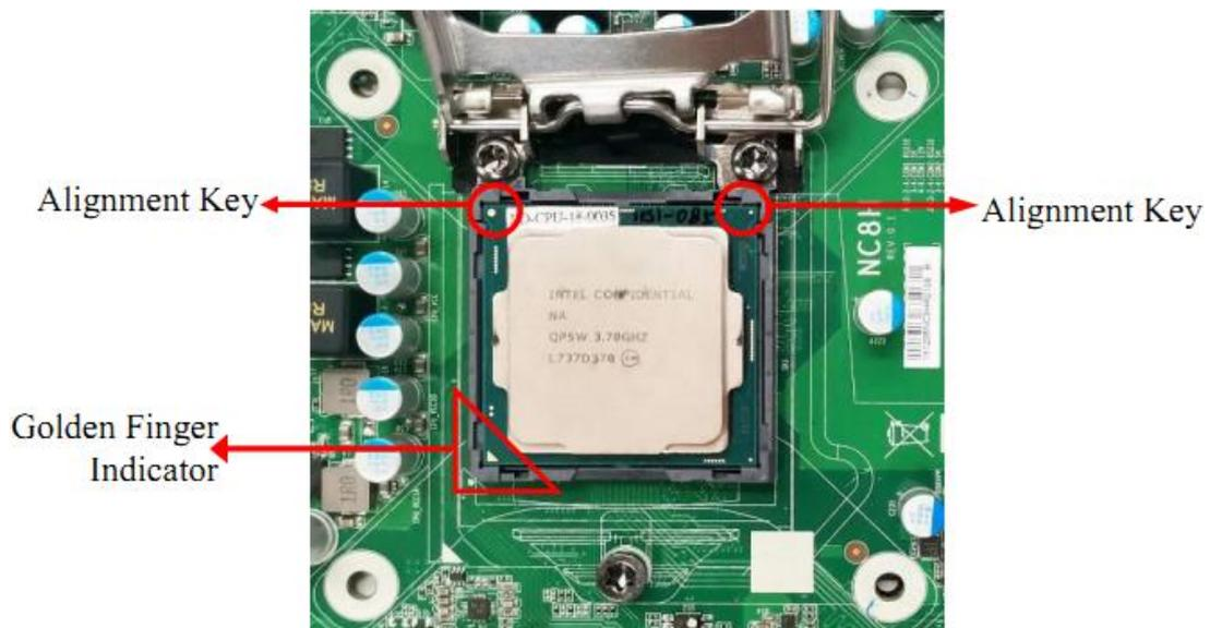
5. Make sure that Pin-1 Golden Finger Indicator in the place as shown in the above photo and match the two alignment keys on the CPU with two points of the socket. CPU can only be correctly installed in this direction. Incorrect installation might cause damage to CPU.
