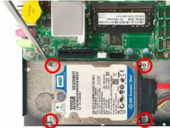
7. Lock the racks hard disk with SATA HDD installed to its original places by tightening the screws in the marked spots.
