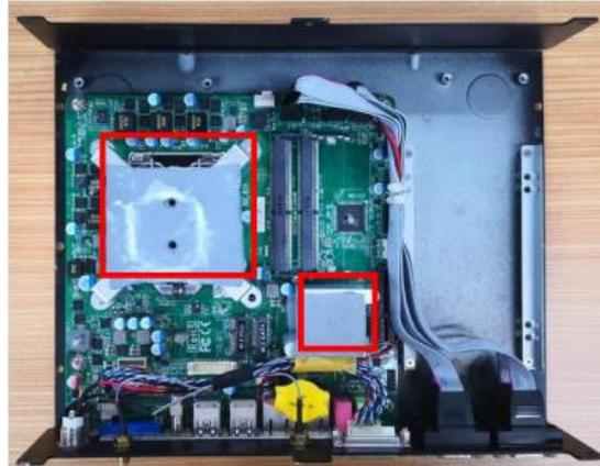
2. Lock the CPU heatsink upon the installed CPU by tightening up the marked screws. The screw holes of the heatsink should match corresponding screw holes of the board.
