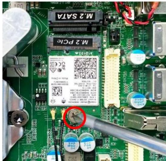
9. Press the metal hats of the antenna string ends to the antenna slots on the card as showed.
