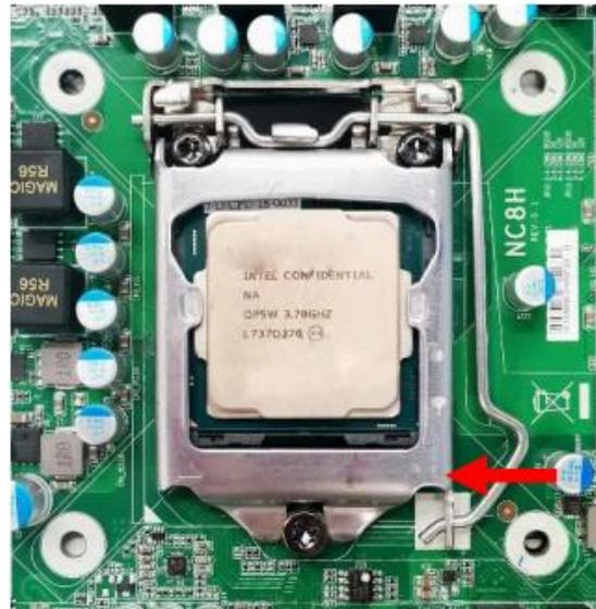
6. Put down the load plate in the direction shown above.
