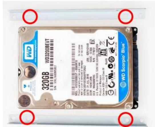
1. Remove the HDD racks from the cover by unscrewing the screws in the marked places.
