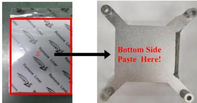
1. Find the above CPU heatsink and CPU thermal grease package. Remove the protective films on the both sides of the grease and apply the grease upon the heatsink for better heat conduction. Apply the grease to the bottom side and the top side of the heatsink at first.
