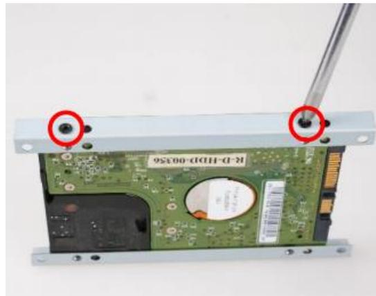
3. Lock the SATA hard disk to one of the racks by tightening the screws in the marked spots.
