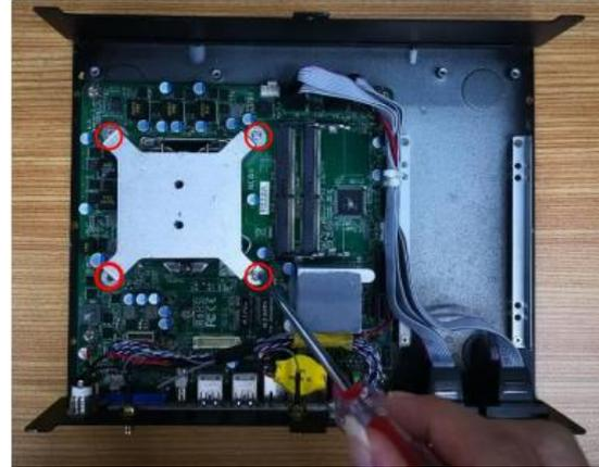
6. Remove the heatsink side cover from the chassis for further installation.
