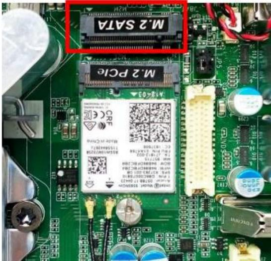
1. Locate the M.2 SATA type-2242 slot on the board.
