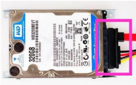
6. Plug this side of the cable to SATA power-in connector and SATA connector of the hard disk.
