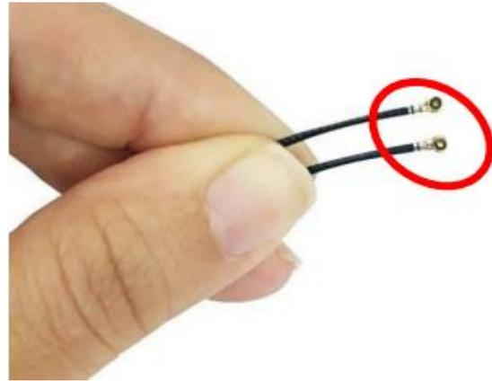
7. The metal hats on the end of the antenna string are sealed by acetate tape to avoid possible damage to the system.
