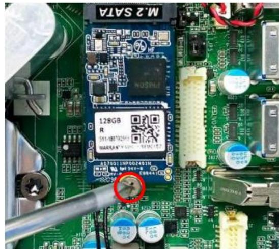
4. Lock the card to the board by tightening up the previously-removed screw to the marked spot.
