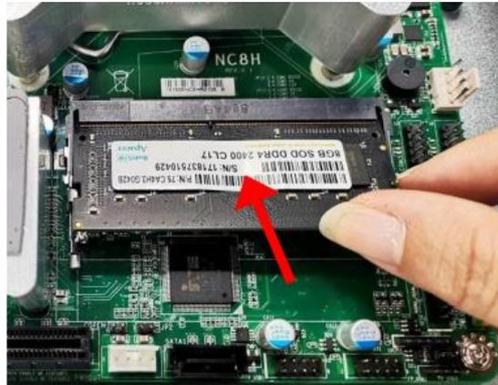
1. Find the SO-DIMM slot on the board for further installation.
