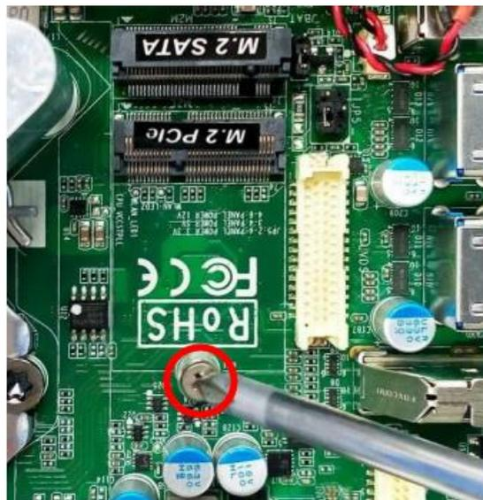
1. Locate the M.2. PCIe, type-2230 slot on the board.
