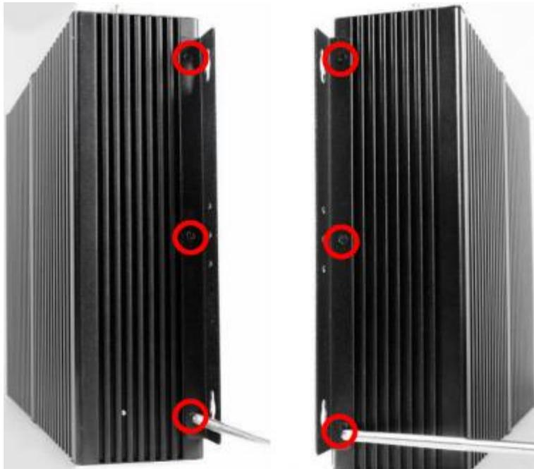
1. Install wall mount rack to the system by tightening the screws in the marked position. Then lock the other three screws on the other side in the same way.
