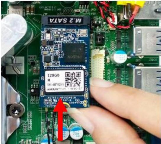
3. Insert the gold-figure side of the compatible M.2 SATA card into the slot. Make sure that the golden-figure side is fully inserted into the slot.
